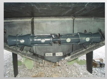
Mounting only 80 mm below the waterline with only four screws
